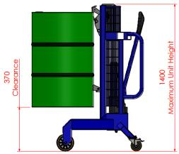
Below is a plan view showing a 200-litre drum being removed from a 1200mm x 1200mm pallet using the DTP05 Corner Depalletiser:
